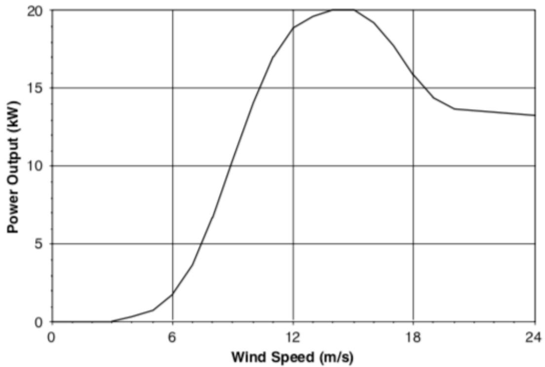
**Figure 15.13** Sample wind turbine power curve.
