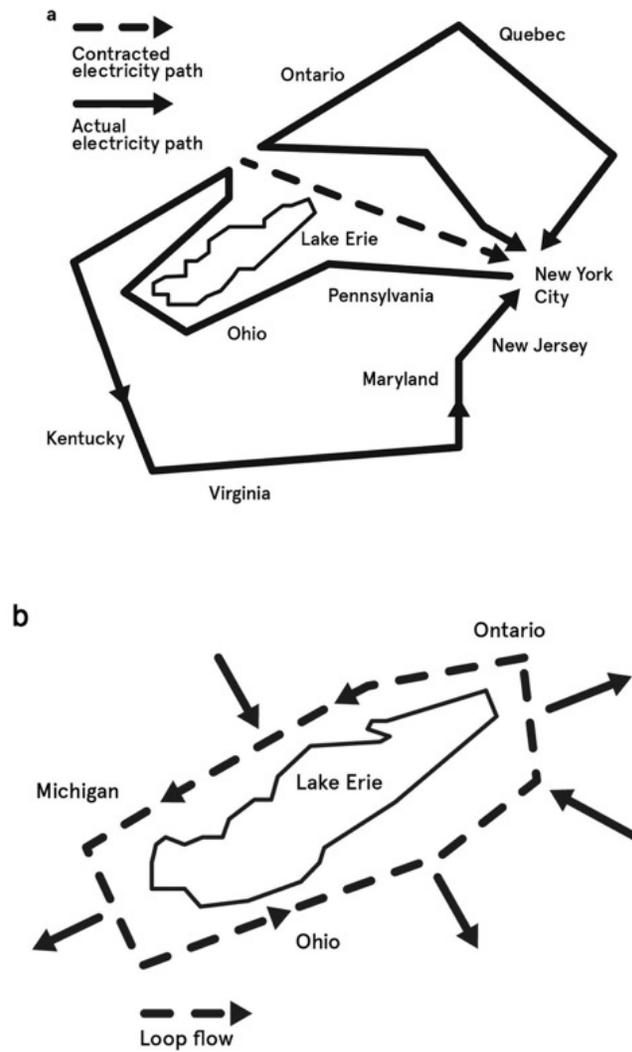
**FIG 4** Electric power does not travel just by the shortest route from source to sink (*top*), but also by parallel flow paths through
