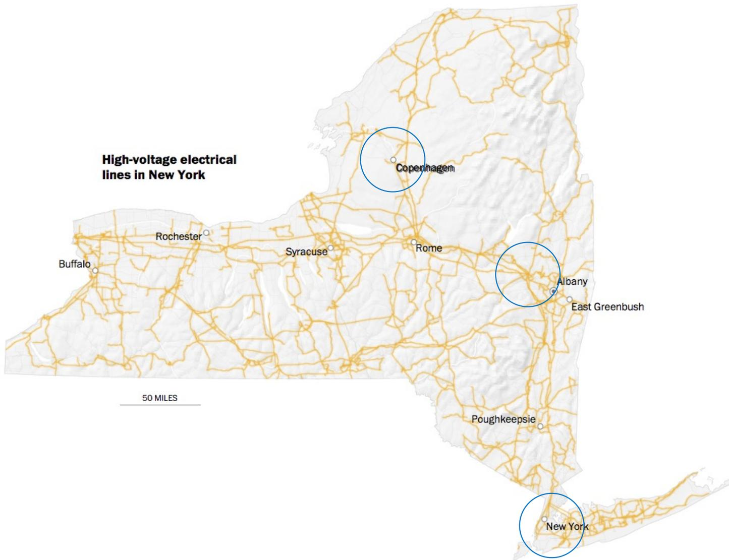
One main transmission line connects the two grids, carrying power from the north and west to where it's needed downstate, which uses about two-thirds of the state's overall energy. Running roughly between Utica and Albany, that line is called the Central East Constraint, and it is congested about half the year, meaning no more power can flow along it.
