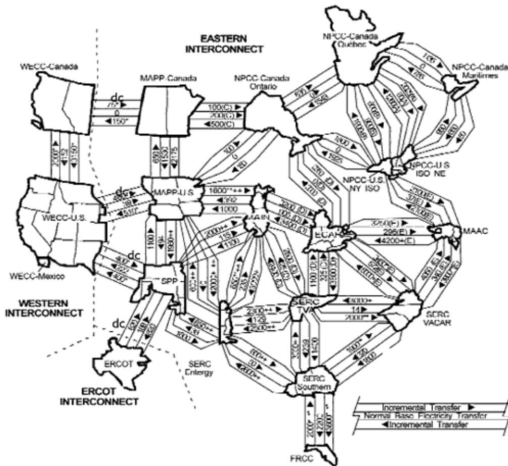
**Figure 1.** Normal U.S. base electricity transfers and first-contingency incremental transfer capabilities, in MW. Credit: North American Electric Reliability Council
