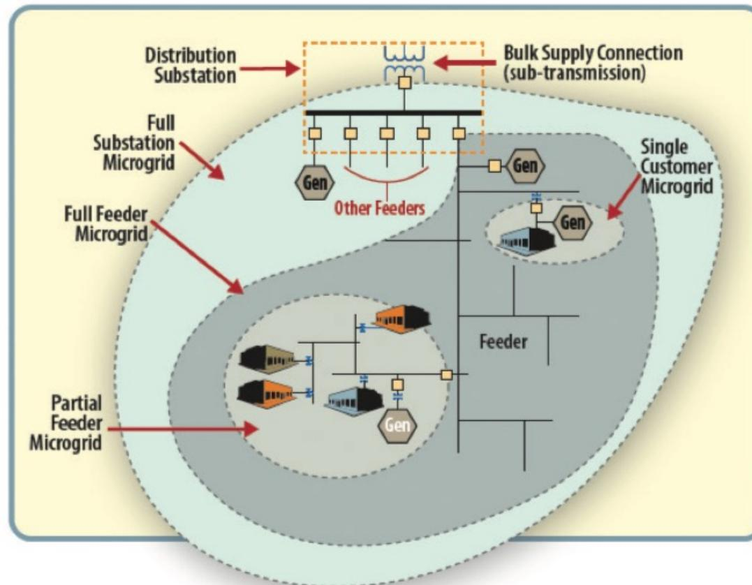
Microgrids can exist in multiple configurations: independently, networked along a feeder, or nested within another.
